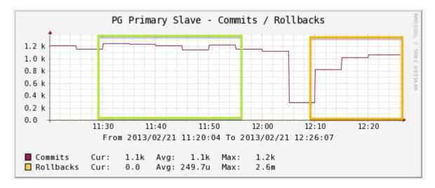
Figure 6 Improved throughput with integrity features enabled (orange rectangle)
