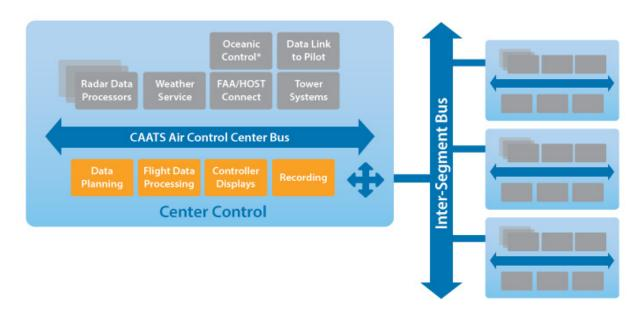
Figure 10. The CAATS integrates centers, communicates to external systems, and links segments together. Intra-center integration (green boxes) will be operational on RTI Connext DDS in 2015.
