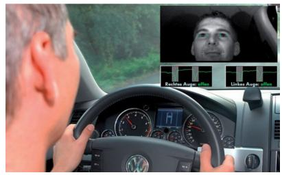
Figure 11. Volkswagen's driver assistance and integrated safety system uses Connext DDS to combine radars, laser range finders and video to assist safe operation. It tracks the driver's eyes to detect drowsiness. It also detects lane departures, avoids collisions and helps keep the car in its lane.
