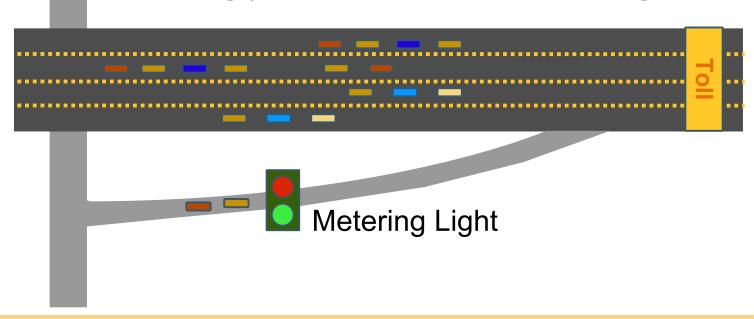
Commuter Highway Uses Access Control via Metering Lights to Maintain Traffic Flow—or Throughput
