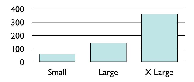
The average speed in writing an 11GB file to /mnt. Large and XLarge instances used software RAID (striping). Full disclosure TBA on http://tocker.id.au/ in April 08.
