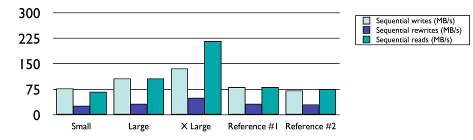
All tests performed on /mnt, with software RAID. Reference #1 system was an Athlon XP 2500+ with a single 10,000 RPM SATA disk. Reference #2 was the same system with a single 7200RPM disk. Full disclosure will be on http://tocker.id.au/ in April 08.
