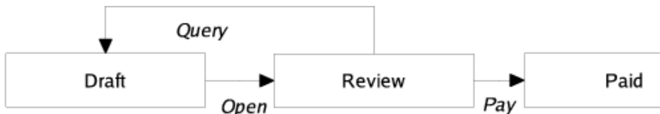
Figure 8-1. A simple state machine for paying credit card bills
