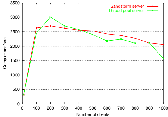
Figure 11: Simple HTTP Server Throughput: This graph shows the performance of a SEDA-based HTTP server implemented using Sandstorm, and a thread pool based server using blocking I/O. The Sandstorm server consists of a single application stage with one thread, while the threaded server has a fixed pool of 150 threads.
