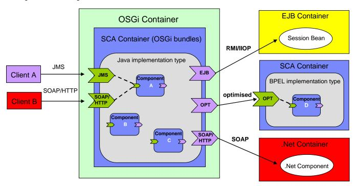
Figure 5: Combined OSGi/SCA Container as part of wider SCA Domain
