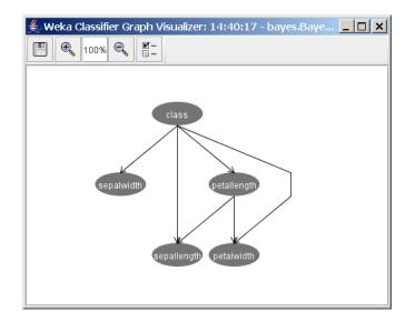
This picture just shows the network structure of the Bayes net, but for each of the nodes a probability distribution for the node given its parents are specified as well. For example, in the Bayes net above there is a conditional distribution for petallength given the value of class. Since class has no parents, there is an unconditional distribution for sepalwidth.
