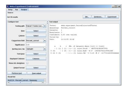
In this experiment, the first row  $(-1\ 1)$  indicates that column b (OneR) is better than row a (ZeroR) and that column c (J48) is also better than row a. The number in brackets represents the number of significant wins for the column with regard to the row. A 0 means that the scheme in the corresponding column did not score a single (significant) win with regard to the scheme in the row.
