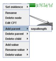
The popup menu shows list of parents that can be deleted from selected node. CPT of the node keeps only the one conditioned on the first value of the parent node.
