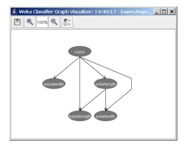
This picture just shows the network structure of the Bayes net, but for each of the nodes a probability distribution for the node given its parents are specified as well. For example, in the Bayes net above there is a conditional distribution
