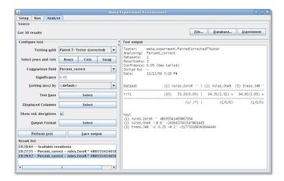
Selecting  $Number\_correct$  as the comparison field and clicking  $Perform\ test$  generates the average number correct (out of 50 test patterns - 33% of 150 patterns in the Iris dataset).
