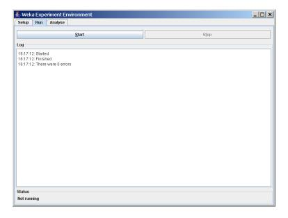
If the experiment was defined correctly, the 3 messages shown above will be displayed in the *Log* panel. The results of the experiment are saved to the dataset *Experiment1.arff*.
