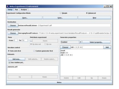
In this experiment, the ZeroR, OneR, and J48 schemes are run 10 times with 10-fold cross-validation. Each set of 10 cross-validation folds is then averaged, producing one result line for each run (instead of one result line for each fold as in the previous example using the *CrossValidationResultProducer*) for a total of 30 result lines. If the raw output is saved, all 300 results are sent to the archive.
