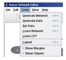
The Generate Network menu allows generation of a complete random Bayesian network. It brings up a dialog to specify the number of nodes, number of arcs, cardinality and a random seed to generate a network.
