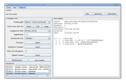
The ranking test ranks the schemes according to the total number of significant wins (>) and losses (<) against the other schemes. The first column (>-<) is the difference between the number of wins and the number of losses. This difference is used to generate the ranking.
