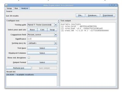
The number of result lines available (Got 30 results) is shown in the Source panel. This experiment consisted of 10 runs, for 3 schemes, for 1 dataset, for a total of 30 result lines. Results can also be loaded from an earlier experiment file by clicking File and loading the appropriate .arff results file. Similarly, results sent to a database (using the DatabaseResultListener) can be loaded from the database.
