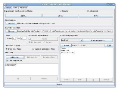
After the experiment setup is complete, run the experiment. Then, to analyse the results, select the Analyse tab at the top of the Experiment Environment window.
