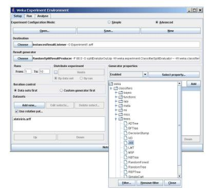
The *Filter*... button enables one to highlight classifiers that can handle certain attribute and class types. With the *Remove filter* button all the selected capabilities will get cleared and the highlighting removed again.
