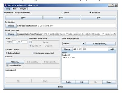
The number of runs is set to 1 in the *Setup* tab in this example, so that only one run of cross-validation for each scheme and dataset is executed.
