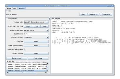
In this experiment, the first row  $(-1\ 1)$  indicates that column b (OneR) is better than row a (ZeroR) and that column c (J48) is also better than row a. The number in brackets represents the number of significant wins for the column with regard to the row. A 0 means that the scheme in the corresponding column did not score a single (significant) win with regard to the scheme in the row.
