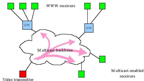
Figure 1. Typical network configuration using gateways
