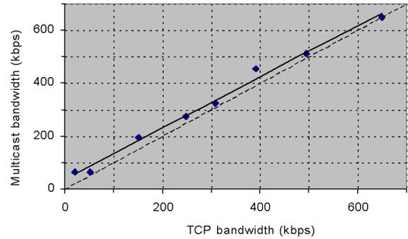
**Figure 4: Multicast bandwidth allocation in relation to HTTP/TCP bandwidth**
