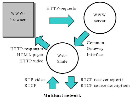
Figure 2: Conceptual model of the WebSmile server architecture
