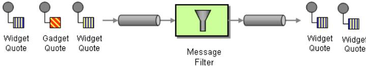
The following example shows how to create a Message Filter route consuming messages from an endpoint called **queue:a** which if the Predicate is true will be dispatched to **queue:b**
