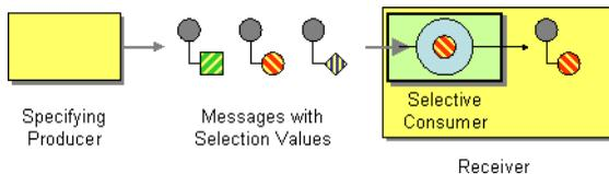
The first solution is to provide a Message Selector to the underlying URIs when creating your consumer. For example when using JMS you can specify a selector parameter so that the message broker will only deliver messages matching your criteria.
