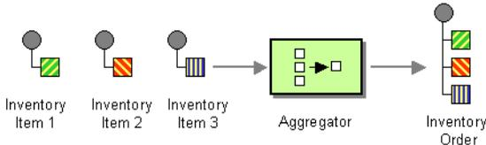
A correlation Expression is used to determine the messages which should be aggregated together. If you want to aggregate all messages into a single message, just use a constant expression. An AggregationStrategy is used to combine all the message exchanges for a single correlation key into a single message exchange.
