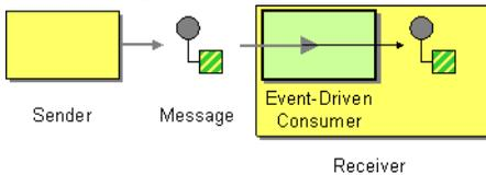
The Event Driven Consumer is implemented by consumers implementing the Processor interface which is invoked by the Message Endpoint when a Message is available for processing.
