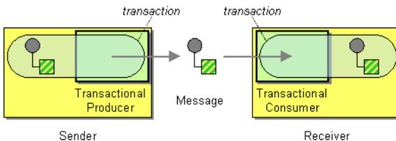
Transaction Oriented Endpoints (Camel Toes) like JMS support using a transaction for both inbound and outbound message exchanges. Endpoints that support transactions will participate in the current transaction context that they are called from.
