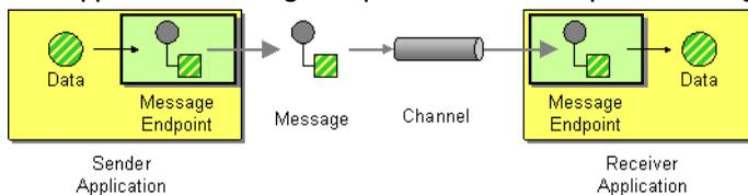
When using the DSL to create Routes you typically refer to Message Endpoints by their URIs rather than directly using the Endpoint interface. Its then a responsibility of the CamelContext to create and activate the necessary Endpoint instances using the available Component implementations.
