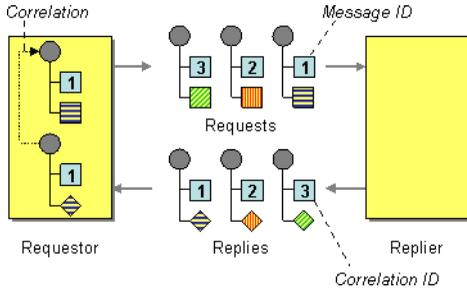
The use of a Correlation Identifier is key to working with the Camel Business Activity Monitoring Framework and can also be highly useful when testing with simulation or canned data such as with the Mock testing framework
