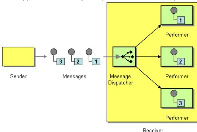
You can use a component like JMS with selectors to implement a Selective Consumer as the Message Dispatcher implementation. Or you can use an Endpoint as the Message Dispatcher itself and then use a Content Based Router as the Message Dispatcher.
