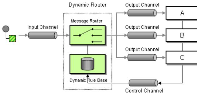
In **Camel 2.5** we introduced a `dynamicRouter` in the DSL which is like a dynamic Routing Slip which evaluates the slip *on-the-fly*.
