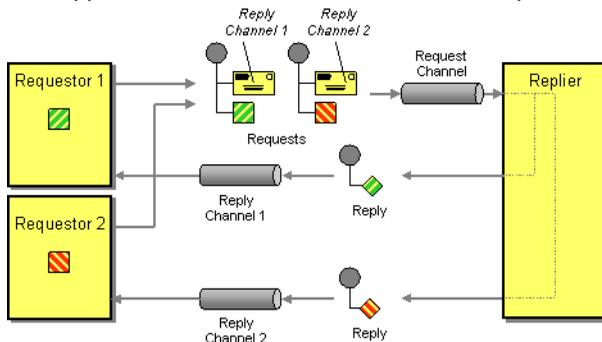
For example when using JMS with InOut the component will by default return to the address given in `JMSReplyTo`.
