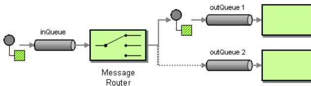
The following example shows how to route a request from an input **queue:a** endpoint to either **queue:b**, **queue:c** or **queue:d** depending on the evaluation of various Predicate expressions
