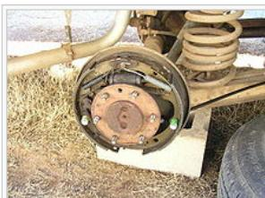
A drum brake with the drum removed, as used on the rear wheel of a car or truck. In this installation, a cable-operated parking brake operates the service shoes.
