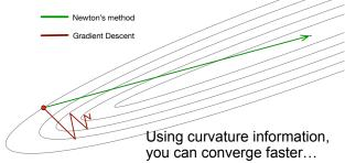
$w_{t+1} \leftarrow w_t - H_t^{-1} g_t$ Exact, impractical  $w_{t+1} \leftarrow w_t - H_t^{-1} g_t$ Using curvature information, you can converge faster...  $d \times d$  matrix of partial derivatives  $\mathcal{O}\left(d^3\right)$  to invert!
