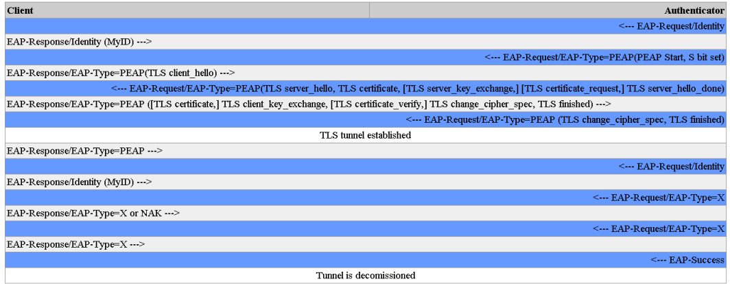
Figure 11 Detailed view of PEAPv1 packet flow
