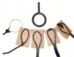
Figure 4.9: Photograph of the loops. The upper one is the EMCO loop. Below from left to right are the nonshielded, symmetrical, balanced and Mariani with and without short.
