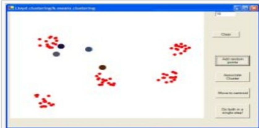
Shows the initial randomized centers and a number of points (actual size here)
