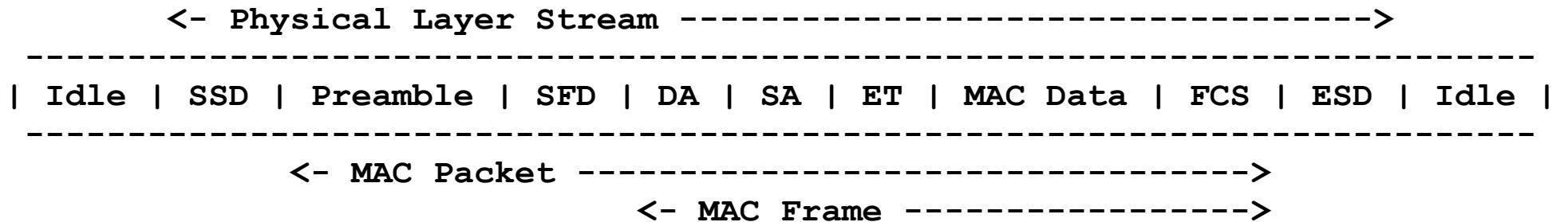
The separation between the PHY and MAC layers requires the transmission of PHY signalling data to be unambiguously encapsulated in relation to the MAC Frame.
