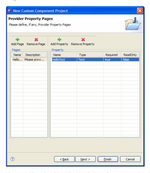
The Pages table on the left is used to identify the configuration pages that will be displayed in the Component Flow Editor. Most components will probably only need one page, but multiple may be defined. For each page added to the Pages table, a set of properties may be defined in the table on the right. These properties will be used to configure the component at runtime (through WSDL extensions) as well as define what is displayed on the wizard page in the Component Flow Editor.
