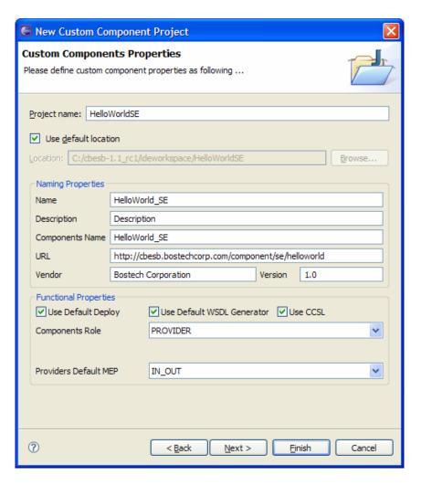
The information in the Naming Properties area is used to identify the component.
