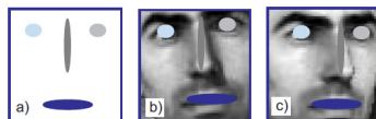
Figure 2. Matching with a set of component templates. The schematic component templates for a frontal face are shown in a). Shifting the component templates can compensate for slight rotations of the face in the image plane b) and in depth c).
