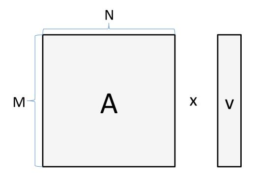
How much data do we need to load from memory? How much data do we need to store to memory? How many FLOPs? 4 bytes  $\times$  (MN + N) 4 bytes  $\times$  M M (2N - 1)  $\approx$  2MN
