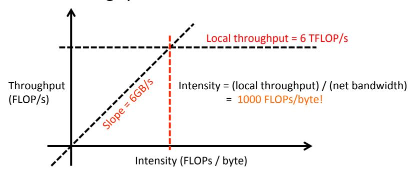
Note much higher intensity: need to do 1000 FLOPs locally (at 6 TFLOP/s throughput) for every 1 byte of network traffic.
