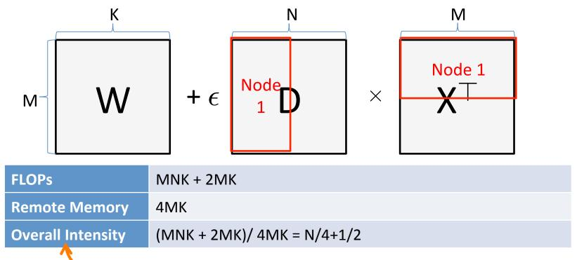
Number of FLOPs we can carry out on Node 1 per byte of network traffic.
