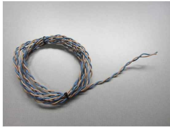
Figure 2-6: 18 gauge twisted pair wire being used for the CAN bus backbone
