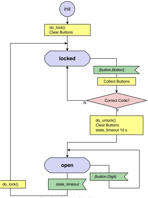
Figure 3.1: Code Lock State Diagram
