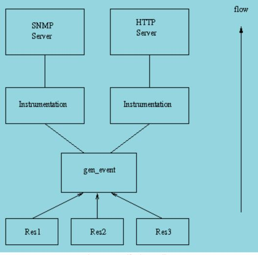
Figure 1.4: Notification Handling
