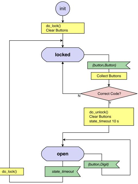
Figure 3.1: Code Lock State Diagram
