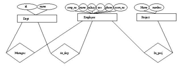
Figure 2.1: Company Entity-Relation Diagram
