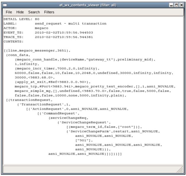
Figure 4.5: The internal form of a Megaco message
