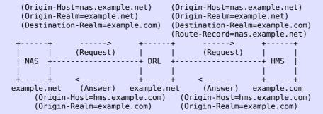
Figure 6: Routing of Diameter messages
