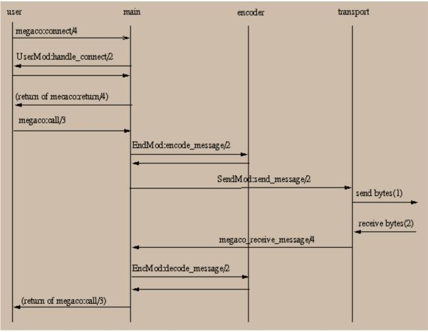
Figure 3.2: MG Startup Call Flow
