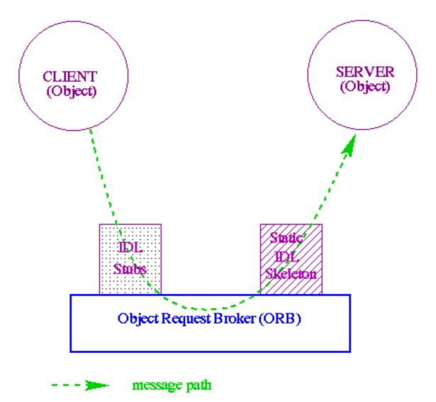
Figure 3.1: Figure 1: How the Object Request Broker works.
