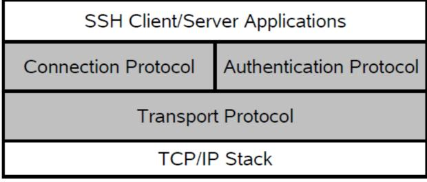
Figure 2.1: SSH Protocol Architecture
