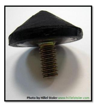
[51.0] Rubber Foot; 1/4-20X1/2inch thread;1inchdiameter 25lb rated
