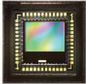
Latest generation CMOS camera 5.6 Gbps
