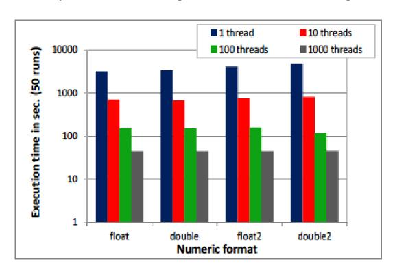
The same tests using the CUMP library exhibit 14x slow-down in case of sequential execution and 500x slow-down when running with 100 threads
