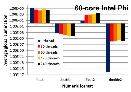
Composite precision outperforms single and double precisions but increasing multithreading makes its accuracy worse
