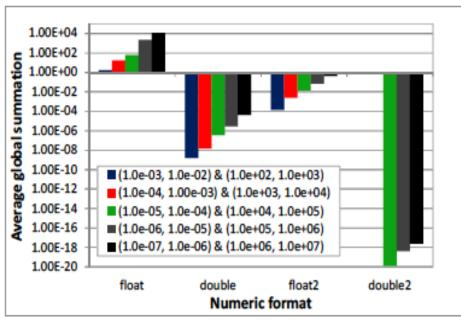
Double precision (double) shows drastic accuracy improvement Composite precision (double2) allows fully accurate results
