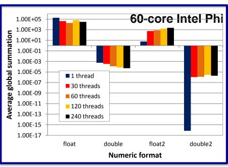
Composite precision outperforms single and double precisions <u>but</u> increasing multithreading makes its accuracy worse
