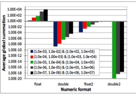
Single precision arithmetic (float) leads to a significant result drift: the computed global summation is as high as 100,000!
