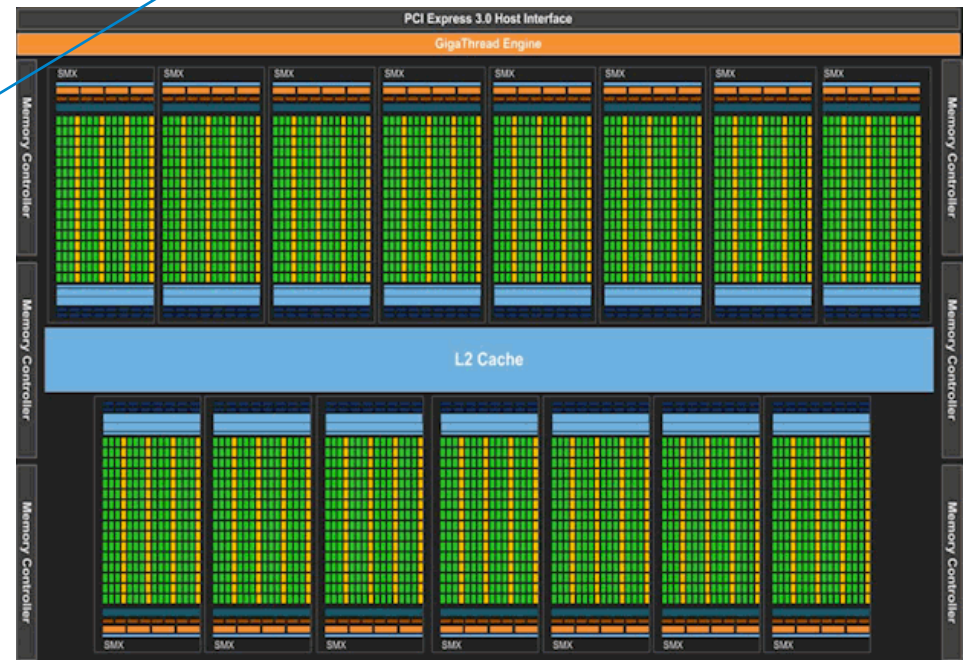
Figure 6. GK110 Logical Layout. On-die memory structures: 1,536KB L2 cache (shared); per-SMX L1 cache (64KB), register file (64Kx32-bit), read-only cache (48KB) Block diagram courtesy NVIDIA Corporation.
