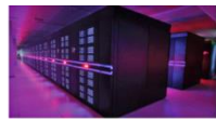
Tianhe-2 (NUDT): TH-IVB-FEP Intel Xeon E5-2692 12 C 2.2 GHz TH Express-2 Intel Xeon Phi 3151P
