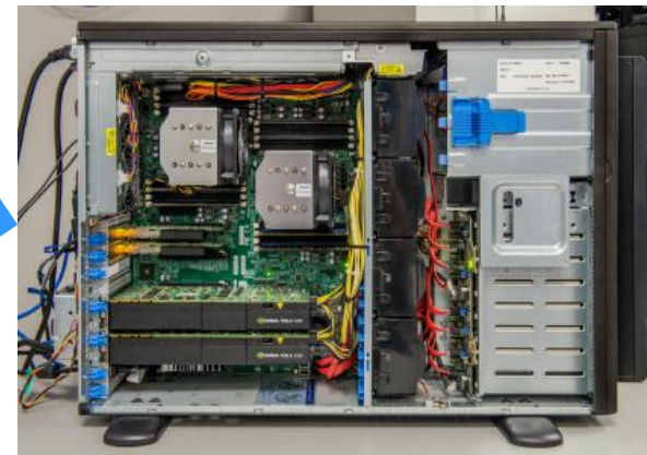
Processing Layer – COTS GPGPUs Perform Bulk of Real-Time Signal Processing with Multi-Core CPU's Completing the Balance
