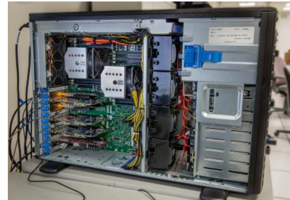
Digitization Layer – COTS A/D Solution Digitizes and Multicasts all CDIF Data to a Scalable Number of Processing Nodes
