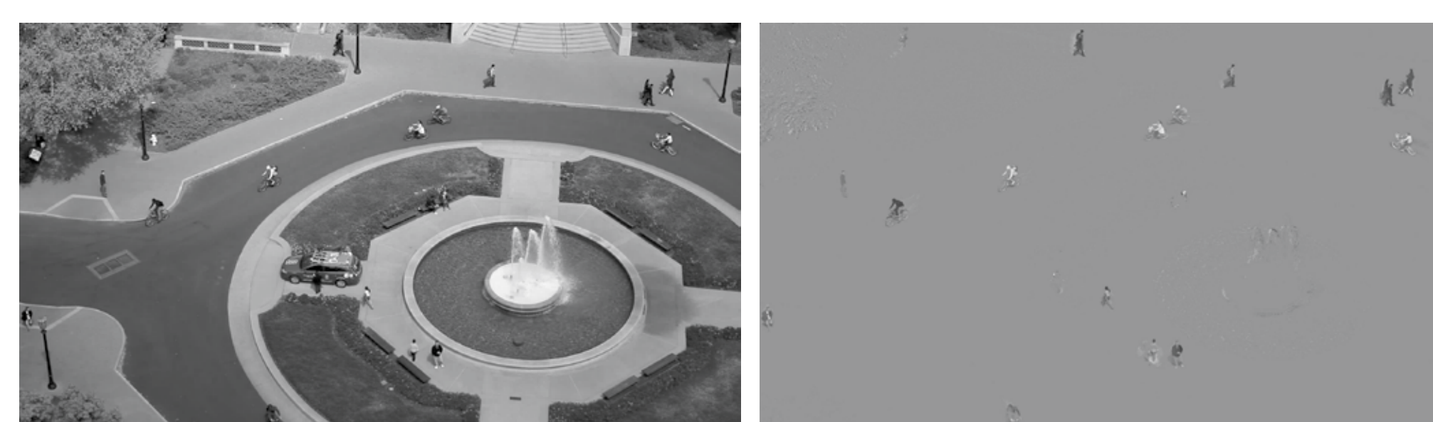
Figure 1: Original frame (160) of the full HD “v1920” test video and corresponding sparse approximation computed on the Jetson TK1 board.
