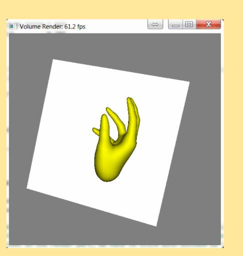
Real-time raycasting of 128<sup>3</sup> signed distance grid computed based on STL model
