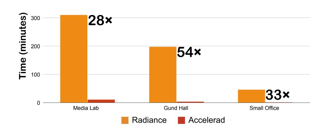
Accelerad shows that ray tracing with irradiance caching and multiple ambient bounces performed on the GPU can be as accurate as traditional Radiance methods for predicting visual comfort conditions in a workplace.
