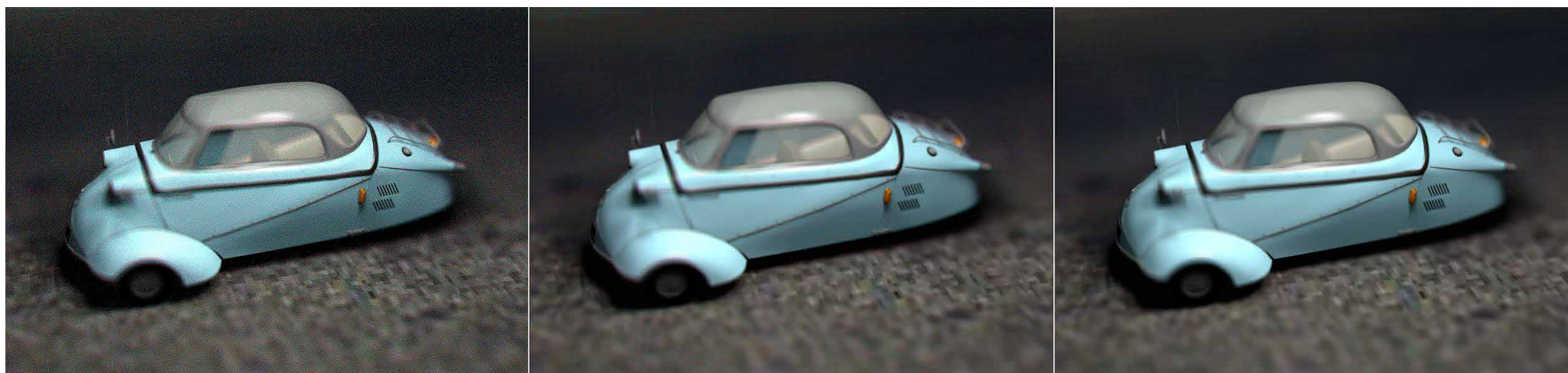
Figure 3: Display simulations. Left: simulated depth of field of binary light field display using 24 red, green, or blue rays per pixel and simple dithering algorithm. Center: Binary light field display with a \sigma = 1 pixel Gaussian low pass filter. Right: Reference image using 24 full color (24-bit RGB) images.
