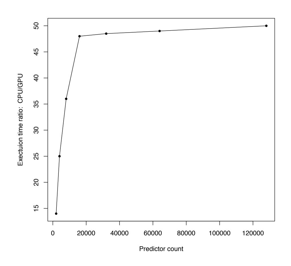
With additional predictors the advantage of the GPU rapidly approaches 50x for this wide example.
