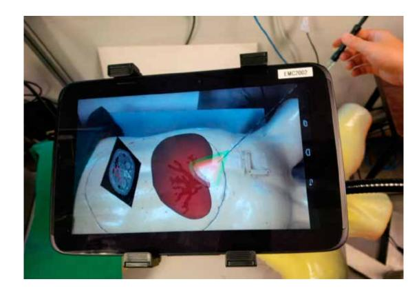
GPU-accelerated registration between point cloud and 3D model
