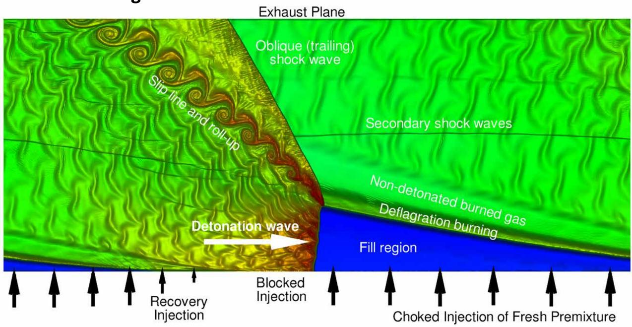
Although the basic operation of an RDE is reasonably well understood, much remains to be learned about its performance, stability of operation, thermal characteristics, and other aspects of operation.
