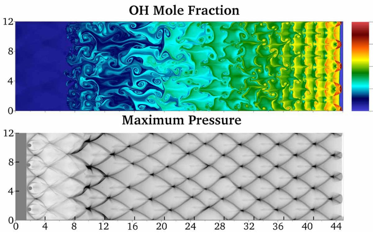
Propel's detailed chemistry solver was benchmarked on a 2D detonation problem (similar to above) with 3.6 million grid cells using a 10 species hydrogen-air mechanism with 34 irreversible reactions. CPUs are 8 core 2.6GHz Intel Xeon E5-2650 v2. GPUs are Nvidia GeForce GTX TITAN Black. The maximum speedup of GPUs relative to CPUs is 6.7. Scalability of GPUs on this problem is limited by the fixed problem size.
