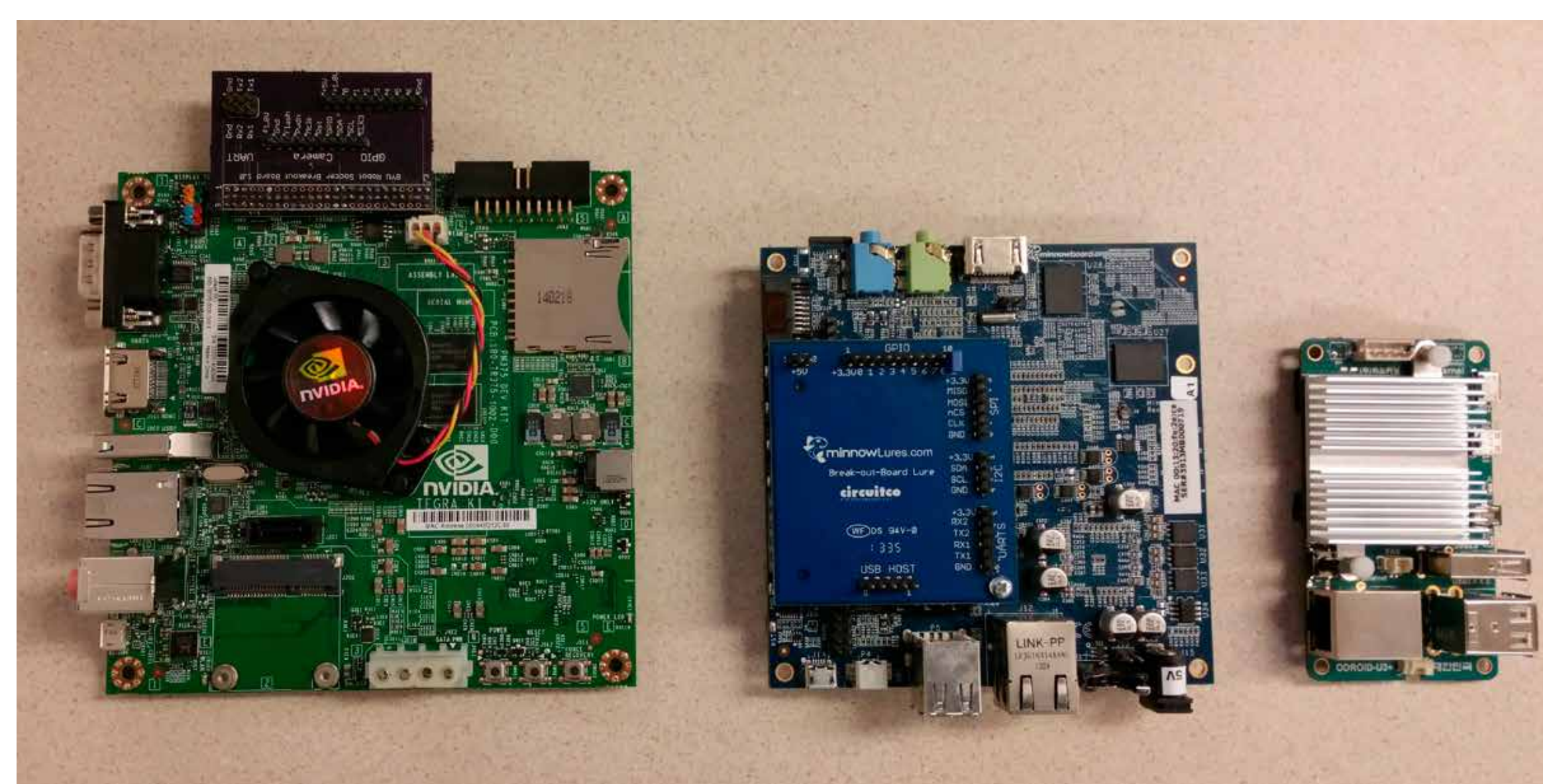
(left to right) Jetson TK1, MinnowBoard, and ODroid U3
