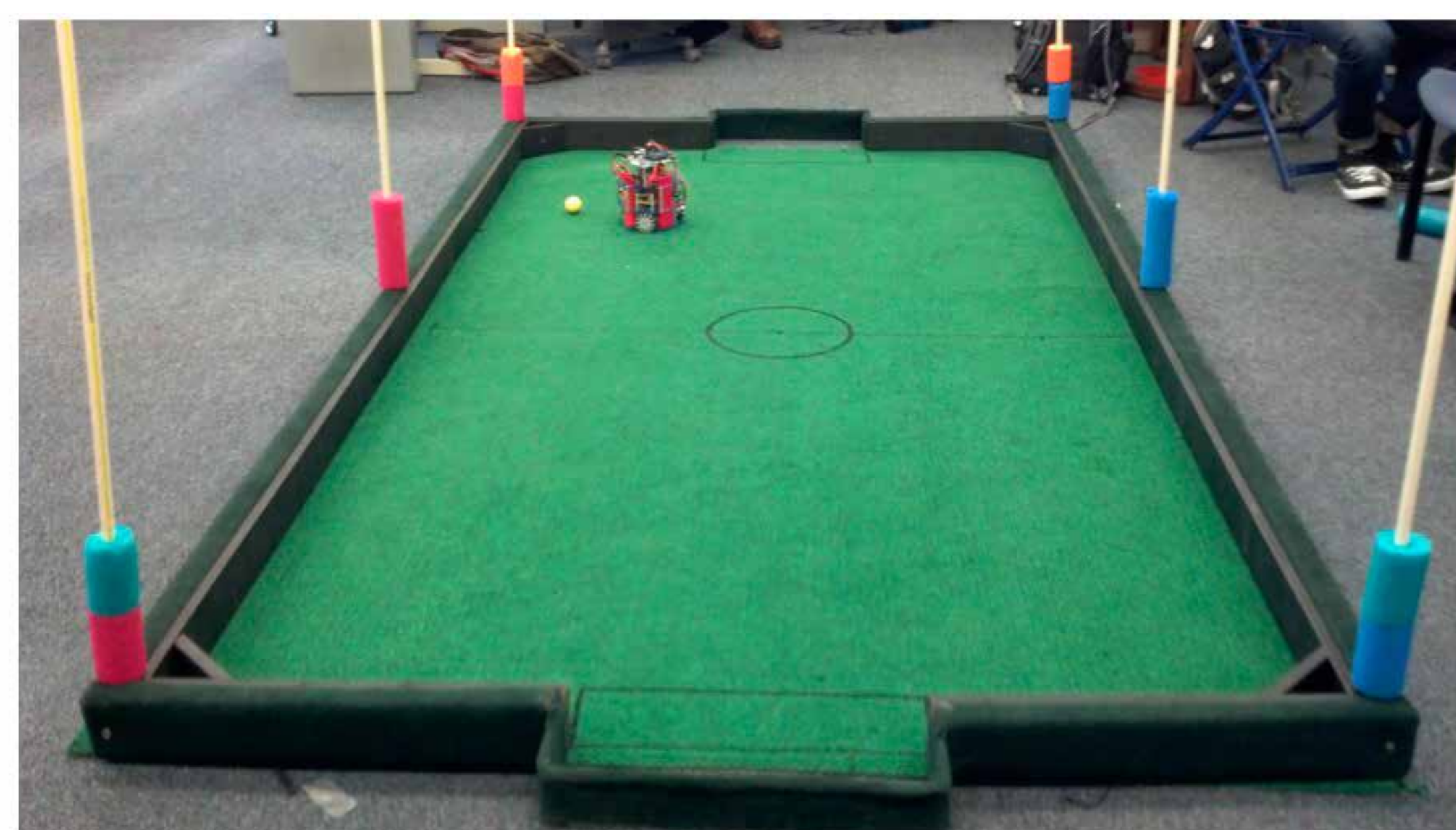
Robot Soccer playing field with markers identifying the corners and midpoint of the field.
