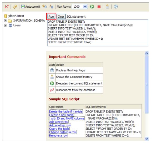
On the left side, a new entry TEST is added below the database icon. The operations and results of the statements are shown
