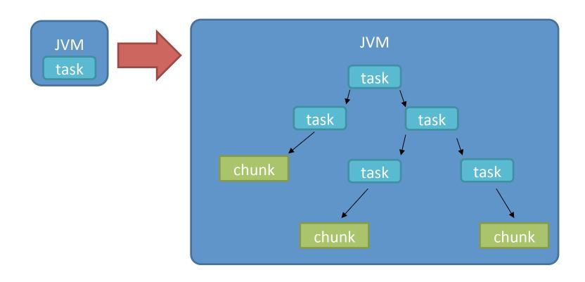
On each node the task is parallelized using Fork/Join
