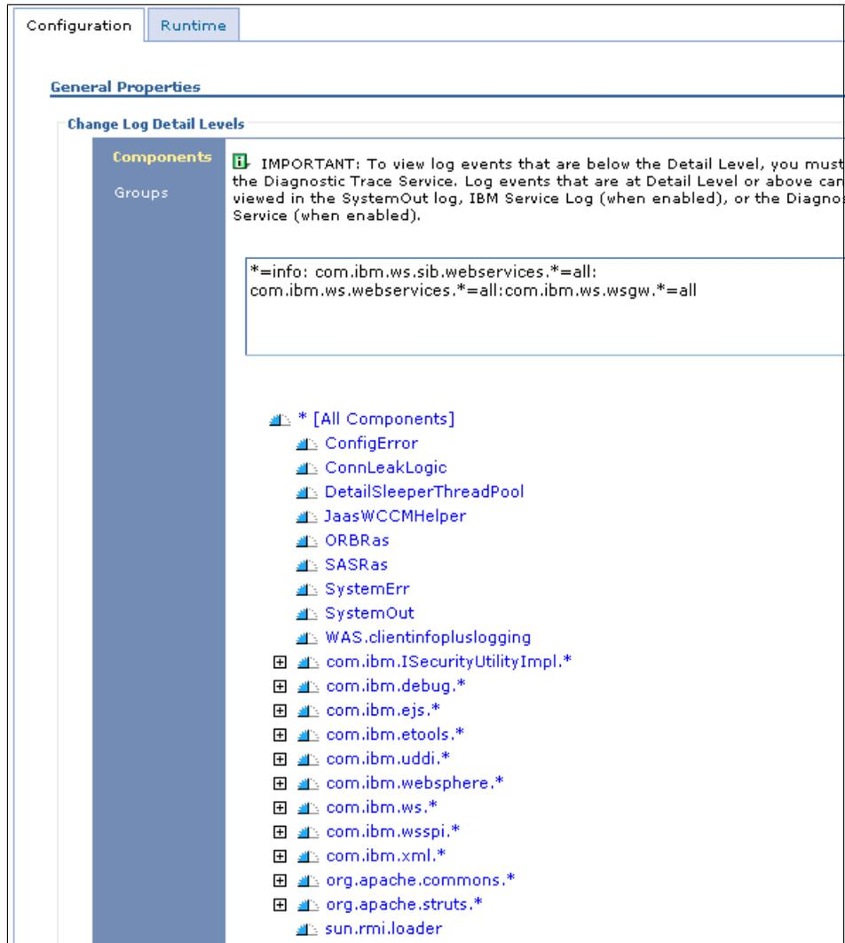
Figure C-5 Enable trace for Web Services Gateway
