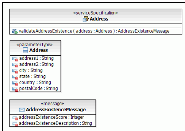
Figure 11-86 Address service specification
