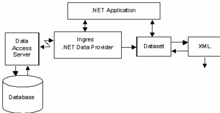
As shown in this figure, the Ingres .NET Data Provider uses an intermediate server called the Data Access Server to access Ingres databases.
