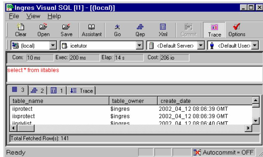
This window allows all the functionality of the previous SQL/Test window in VDBA, but has the following additional toolbar controls:
